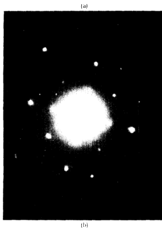
Fig. 3. A Small aggregate of \beta\text{W}_2\text{C} under a transmission electron microscope.
